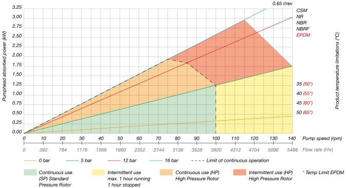
Any application below 15 Hz may require special review. Flows are typical and were measured with water at 20°C with no suction lift or discharge pressure. Actual flows will vary according to suction conditions, discharge pressure and normal component production tolerances.
