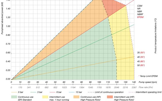
Any application below 15 Hz may require special review. Flows are typical and were measured with water at 20°C with no suction lift or discharge pressure. Actual flows will vary according to suction conditions, discharge pressure and normal component production tolerances.
