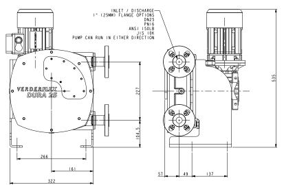
N.B. GMU AND MOTOR SHOWN: -MOTOVARIO NMRVP\_063 WITH FA OUTPUT FLANGE AND 71 FRAME B5 FLANGE MOTOR.
